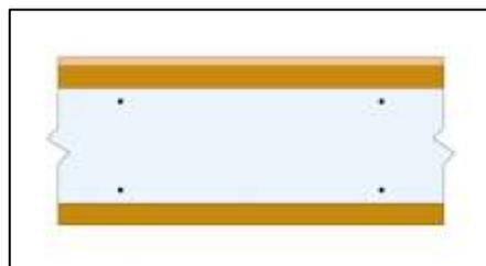
Figure 2a: end view of the installation of 12.5 mm (1/2 in.) regular gypsum board flange-to-flange of I-joist
