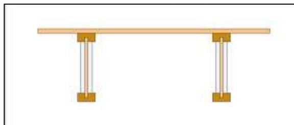
**Figure 1b: side view of the installation of 12.5 mm (1/2 in.) regular gypsum board to protect web of I-joist**
