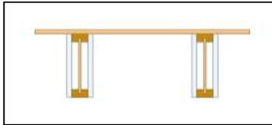
Figure 2b: side view of the installation of 12.5 mm (1/2 in.) regular gypsum board flange-to-flange of I-joist
