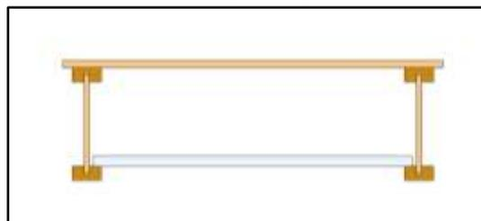
Figure 3b: side view for wood I-joist at 600 mm spacing, placing 15.8 mm (5/8 in.) regular gypsum board on top of bottom flange of I-joist
