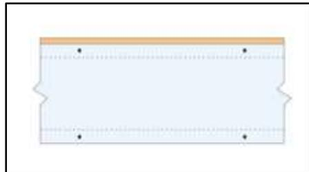
Figure 3a: end view for wood I-joist at 600 mm spacing, placing 15.8 mm (5/8 in.) regular gypsum board on top of bottom flange of I-joist
